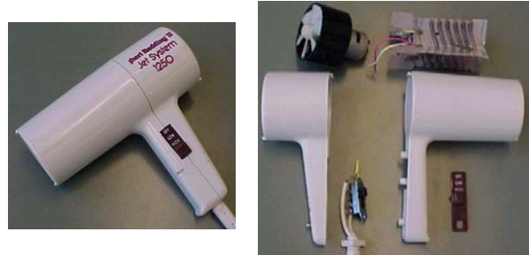
Figure 9: Hair Dryer and its Major Component
